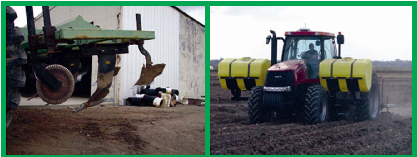
A four row Paratill® subsoiler was used in the demonstration trials for the deep tillage operation conducted in the fall.
