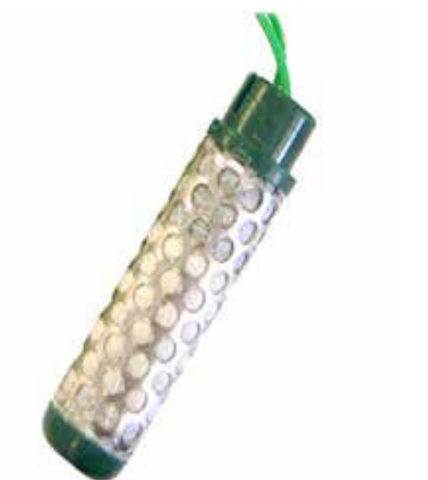
Figure 3. Sensor used to measure infiltration rates.
