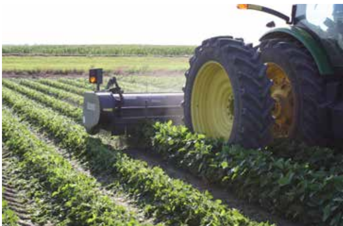
Figure 1 (above). Tractor flail mower used to simulate hail damage in the demonstration trial.
