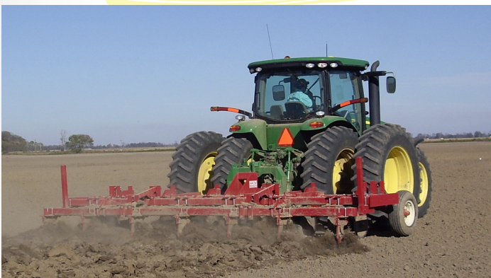
Figure 1. A parabolic subsoiler was used for deep tillage treatments.
