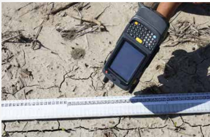
Figure 1. Barcode ruler and Motorola Symbol reader used to record corn plants that emerge and their distribution in the row.
