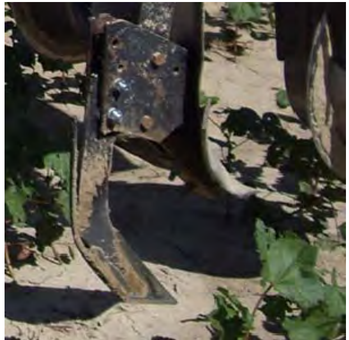
Figures 2 (left) and 3 (above). A subsoiler was constructed with the use of M1 Winged Anhydrous Knives manufactured by Nichols Tillage Tools® mounted on an Orthman® toolbar.
