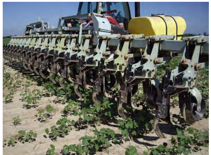
Figure 1. A subsoiler was constructed with the use of M1 Winged Anhydrous Knives manufactured by Nichols Tillage Tools ® mounted on an Orthman ® toolbar.
