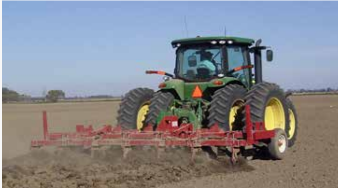
Figure 1. A parabolic subsoiler was used for deep tillage treatments.
