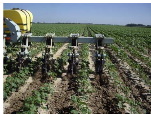
Figure 1 - 3. A subsoiler was constructed with the use of M1 Winged Anhydrous Knives manufactured by Nichols Tillage Tools ® mounted on an Orthman ® toolbar.
