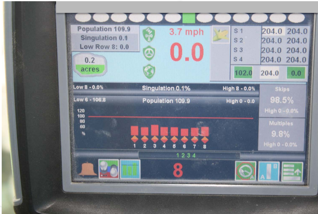
Figure 1. Using predetermined data from a 'skipulator', planters were programmed to randomly insert skips into each planting population.
