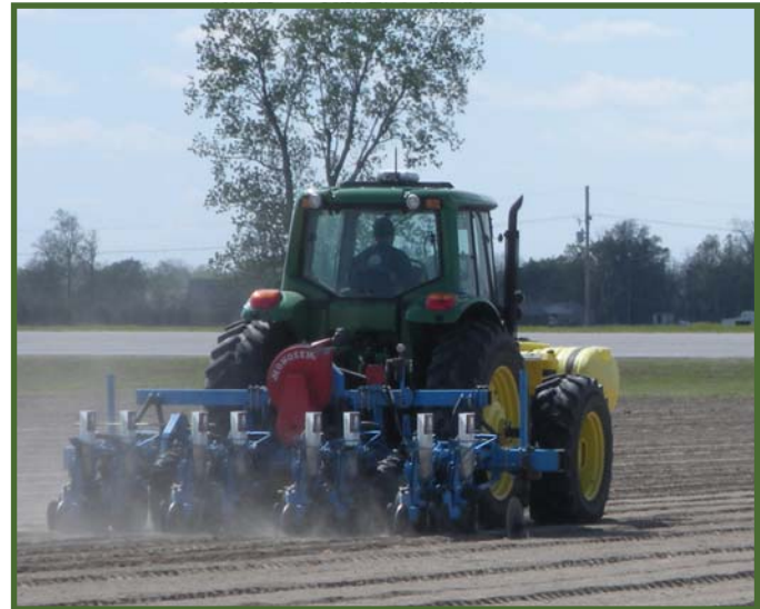
Figure 5. Planting twin rows with Monosem ® planter.
