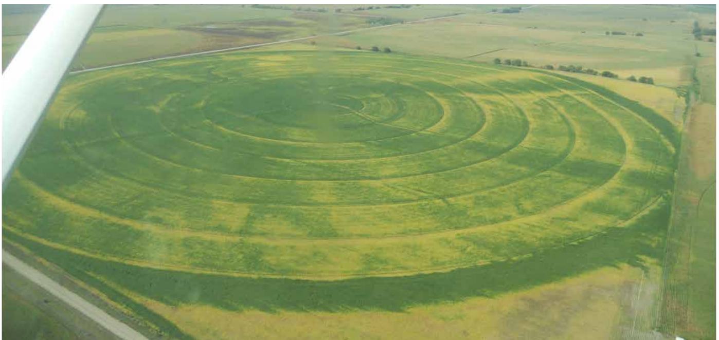
Figure 3.5 Variability in rings under a center pivot may indicate nozzle or other water delivery problems. Photo courtesy of Gary Zoubek, University of Nebraska-Lincoln.
